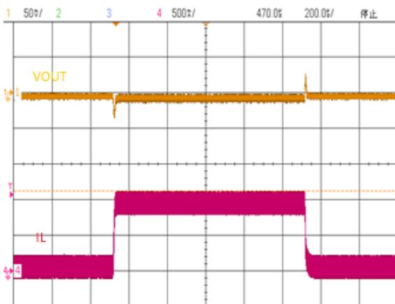
$V_{in}@3.3\text{V}$  Transient ripple at 0.1A~1A
