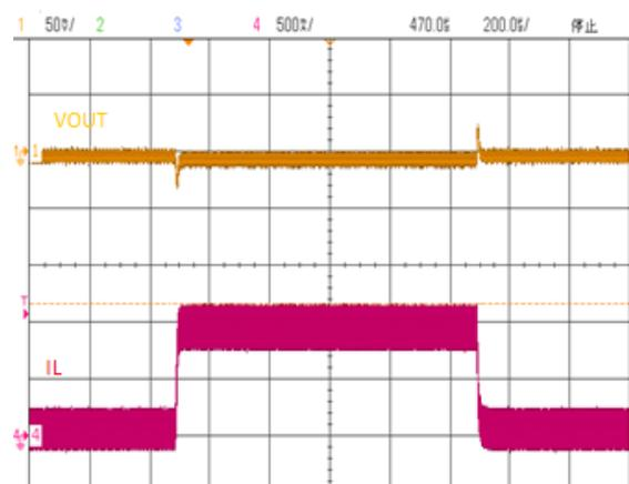
$V_{in}@5\text{V}$  Transient ripple at 1A~0.1A
