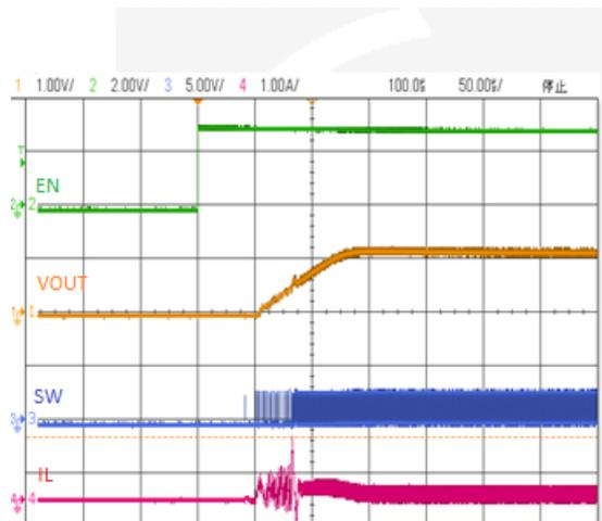
Power-on at  $V_{in}=3.3\text{V}$ ,  $I_{out}=0.1\text{A}$
