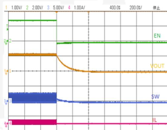
Power-off at  $V_{in}=3.3\text{V}$ ,  $I_{out}=0.1\text{A}$
