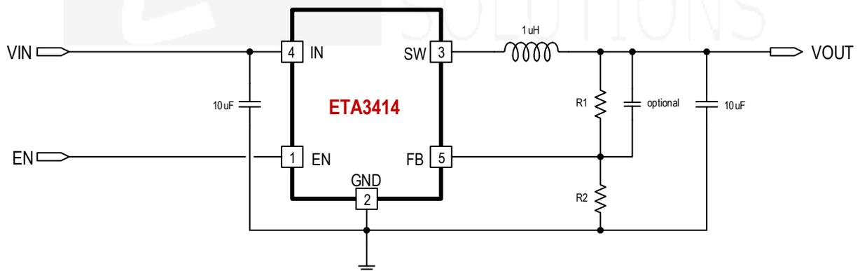
$$V_{out} = \frac{R1+R2}{R2} \times 0.6(V)$$
