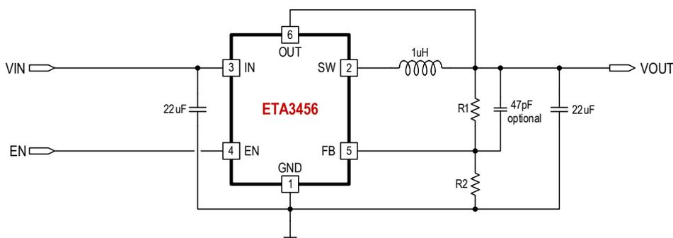
$$V_{out} = \frac{R1+R2}{R2} \times 0.6(V)$$
