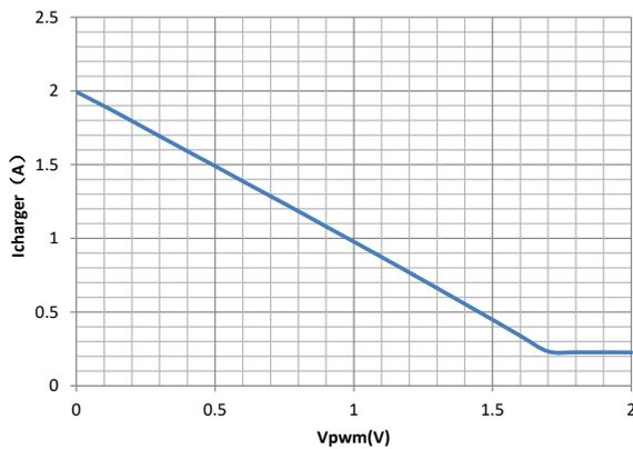
Charge Current Vs.  $V_{pwm}$  at  $R1=220K$ ,  $Rset=130K$
