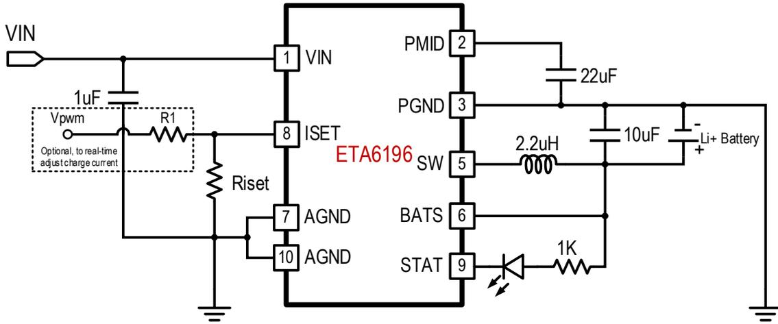
As given by above application circuit, one can real-time adjust the charge current by a PWM signal with different duty-cycle. The  $V_{pwm}$  is the RC filtered voltage of the PWM signal, and it will change linearly with the duty-cycle of the PWM signal. Followings are 2 examples of charge current's relationship to  $V_{pwm}$ . Please contact ETA engineers if one wants to have specific real-time charge current setting, the choosing of  $R1$  and  $Rset$  value will be provided quickly.
