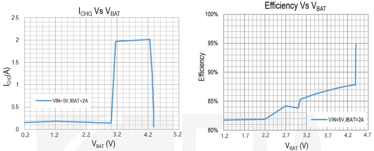
Complete charging cycle of a 10000mAh battery at 2A charge current
