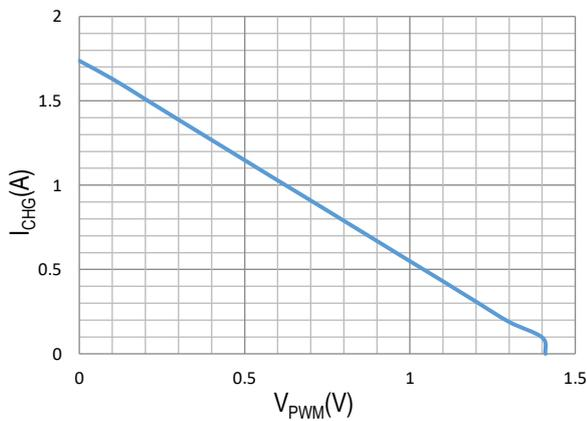
Charge Current Vs.  $V_{pwm}$  at  $R_1=220K$ ,  $R_{ISET}=130K$
