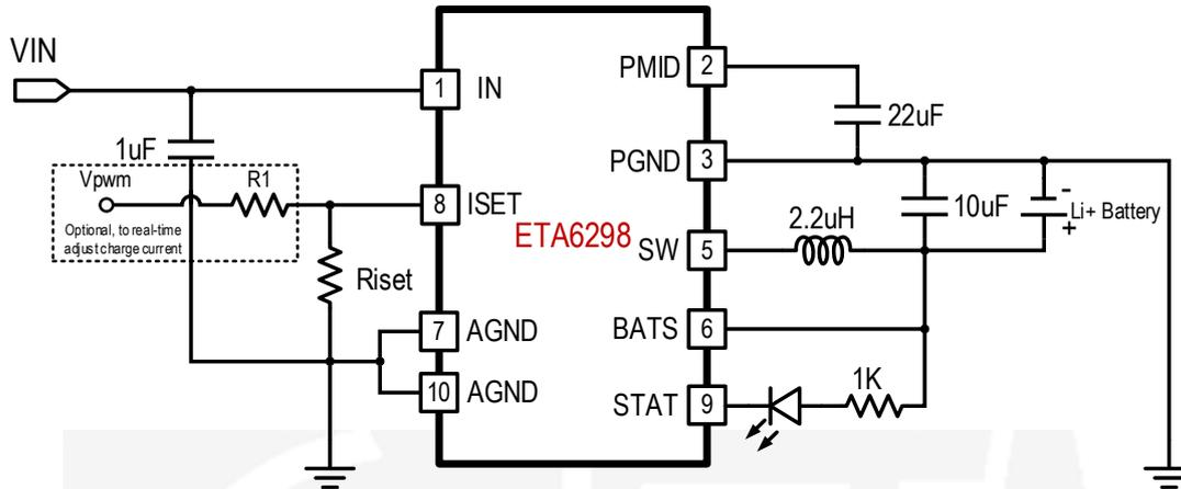
As given by above application circuit, one can real-time adjust the charge current by a PWM signal with different duty-cycle. The  $V_{pwm}$  is the RC filtered voltage of the PWM signal, and it will change linearly with the duty-cycle of the PWM signal. Followings are 2 examples of charge current's relationship to  $V_{pwm}$ . Please contact ETA engineers if one wants to have specific real-time charge current setting, the choosing of  $R_1$  and  $R_{ISET}$  value will be provided quickly.
