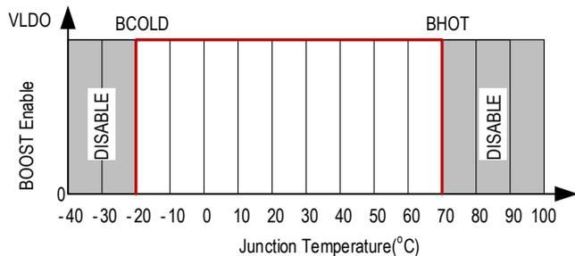
Figure 9: TS Pin Thermistor Sense Threshold in Boost
