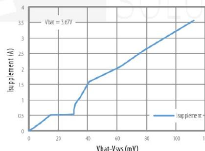
Figure 4: BATFET Current at Entering Supplement Mode
