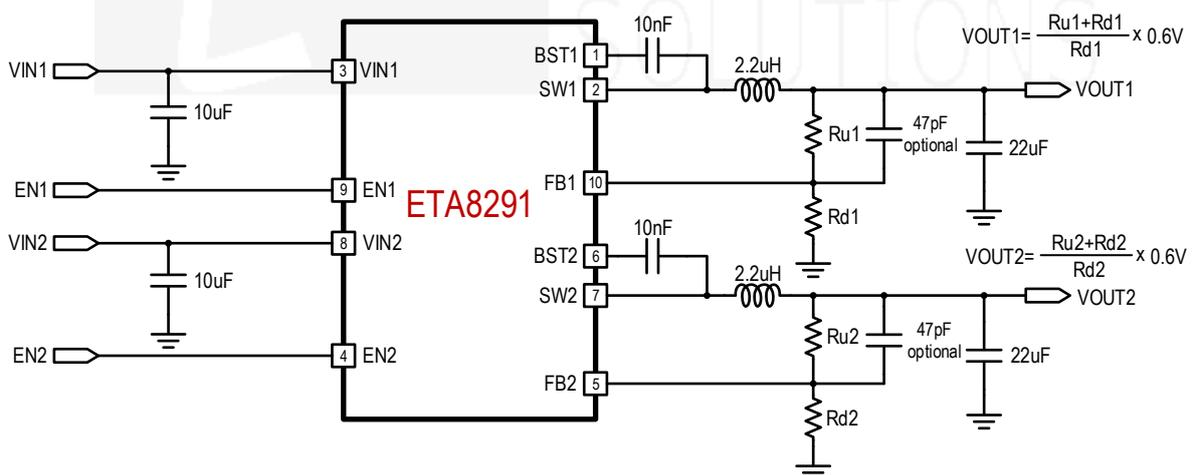
\*Resistors Rd1 and Rd2 have to be between 1KOhm to 70KOhm
