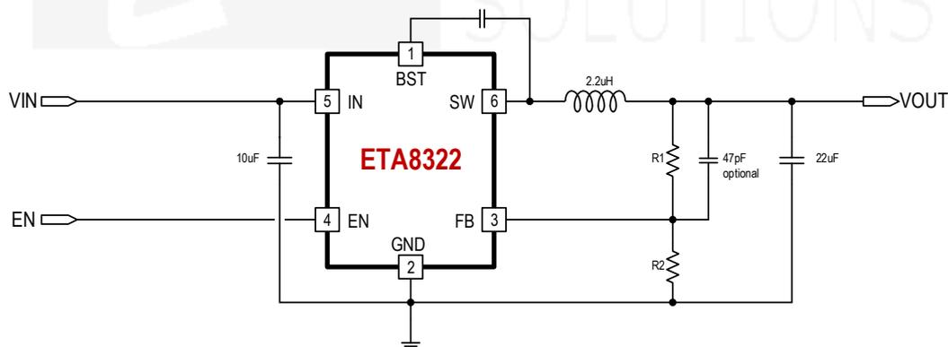
$$V_{out} = \frac{R1+R2}{R2} \times 0.6(V)$$
