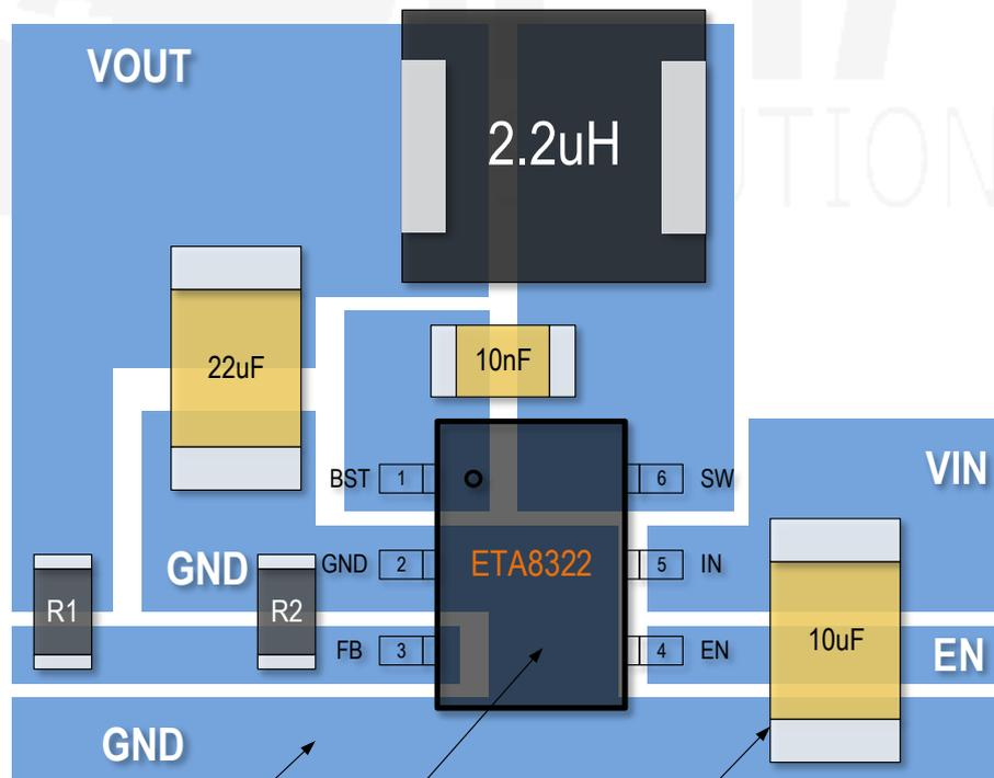
GND trace is used to shield the FB (sensitive node).
