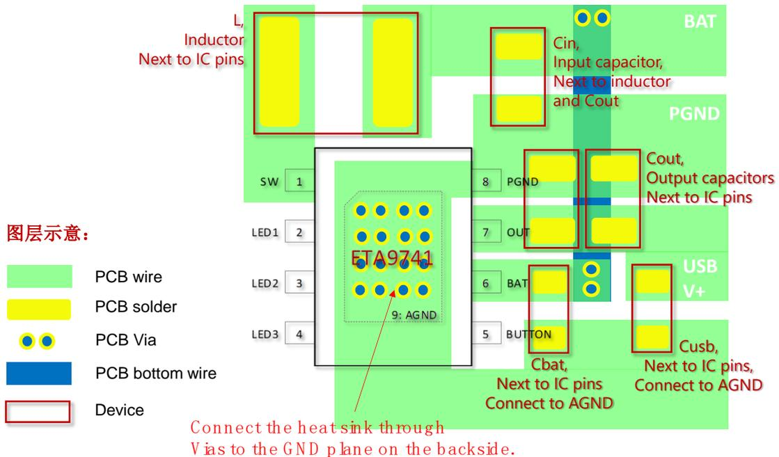
Please have  $C_{IN}$ ,  $C_{OUT}$ , and  $L$  placed just next to the IC pins so that the power traces are kept to the shortest to achieve a good performance of ETA9741 and good EMI.
